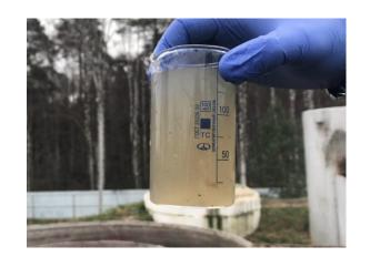
High quality of waste water treatment is confirmed by presence of a sufficiently large and growing number of ciliates and rotifers.
